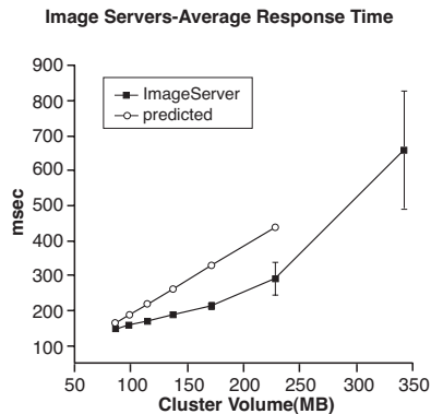
Fig. 9. Declustering effects. The process in which object were cut along their Y - axis and placed in different image servers results in improving the image server's response times when the number of clusters increases
