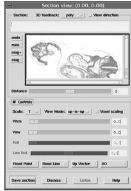
Fig. 1. GUI to process 3D Woolz images. Specialized components enable the rotation within the 3D space. The requested sections can be scaled, magnified and saved to disk
